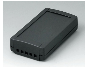
B1055469 TOPTEC 123 F, Vers. II ABS (UL 94 HB) black RAL 9005 123x68x30mm IP 40
