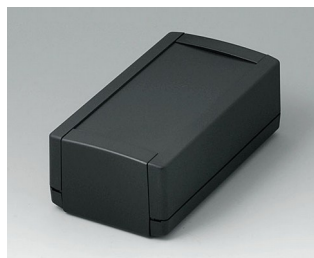
B1060369 TOPTEC 154 H, Vers. I ABS (UL 94 HB) black RAL 9005 154x84x56mm IP 40
