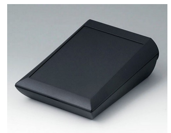
A0615109 COMTEC 150 H, Vers. I ABS (UL 94 HB) black RAL 9005 150x200x71.5mm IP 40
