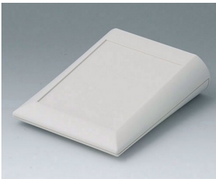
A0612007 COMTEC 120 F, Vers. I ABS (UL 94 HB) off-white RAL 9002 120x150x42.8mm IP 40
