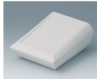
A0612107 COMTEC 120 H, Vers. I ABS (UL 94 HB) off-white RAL 9002 120x150x62.8mm IP 40
