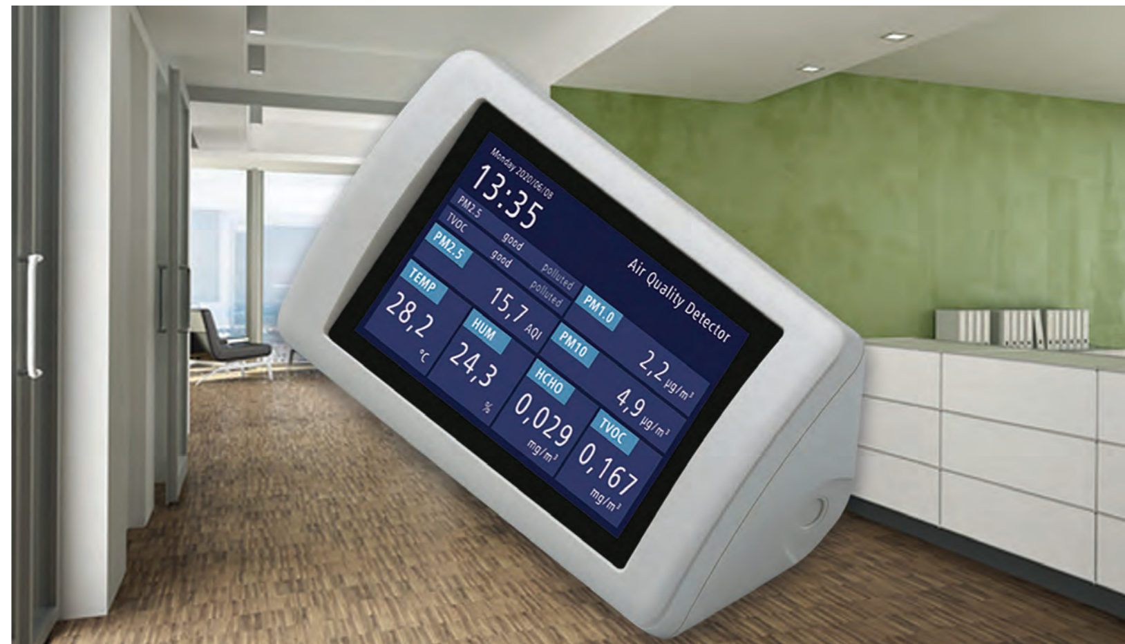
SMART-CONTROL for testing air quality in enclosed spaces
