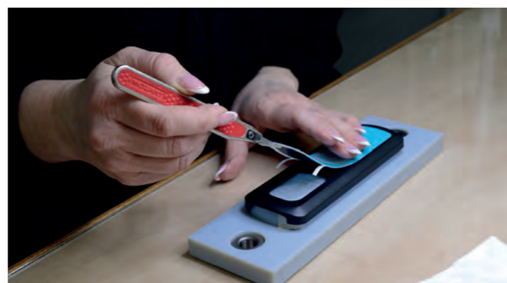
Gluing the front foil to the enclosure
